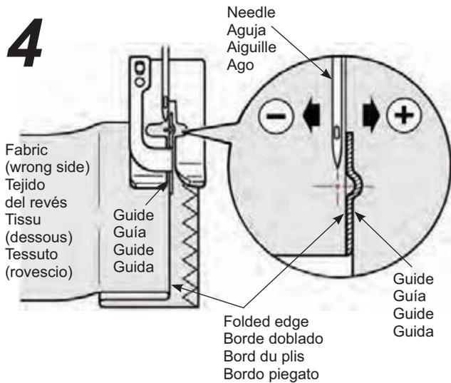
● **Align the guide of the presser foot with the folded edge.**
