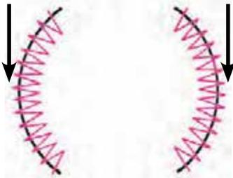
Keep the needle inside the fabric at the point of arrow and raise the presser foot.
