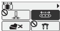
The twin needle setting can only be carried out when suitable pattern is selected and center needle position is selected at the same time.
