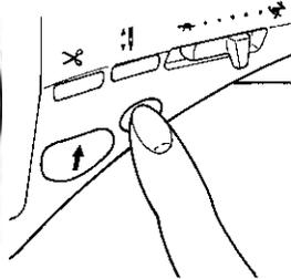
● **When the machine comes to the sewing end point, push the reverse stitch button.**
