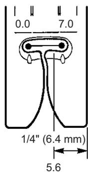
The needle position can be adjusted between 0.0~7.0.
