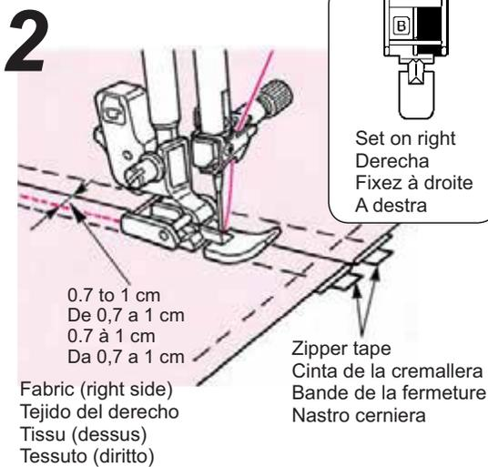
● **Sew the left part of the zipper on the seam allowance from the bottom of the opening to the top.**
