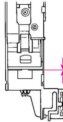
If there is not a clearance, the machine will not sew neat stitches.
