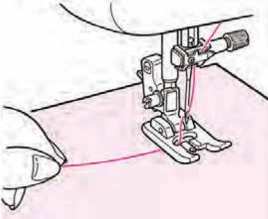
**Place the fabric underneath the presser foot and start.**
