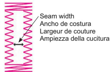
The seam width of buttonhole is changeable. \* It is changeable when sewing a buttonhole.
