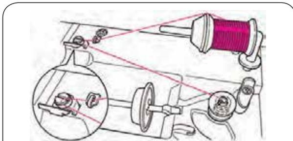
\* Bobbin winding is also possible with supplementary spool pin.
