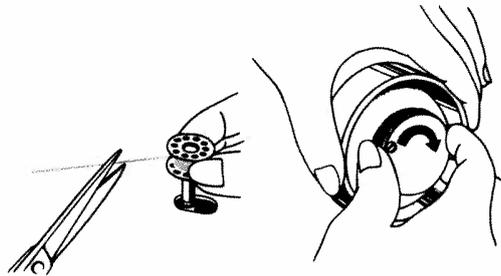
If bobbin is wound unevenly as shown, open face cover and loosen set-screw of the guide for bobbin winding, by using screw driver and adjust height.
