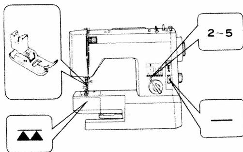
Position a button and material under foot. When needle comes to left side of stitch, lower foot. Raise needle and adjust zigzag width so that needle comes to right hole of button.
