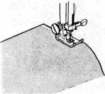
Release lever and commence forward sewing guiding fabric by hand as it is fed.
