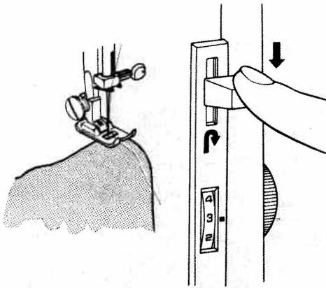
To reinforce seam, sew backwards to the edge of fabric by pushing down reverse sewing lever.
