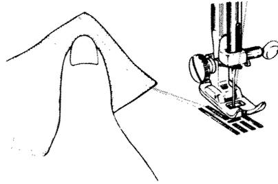
Cut threads with thread cutter behind presser bar.
