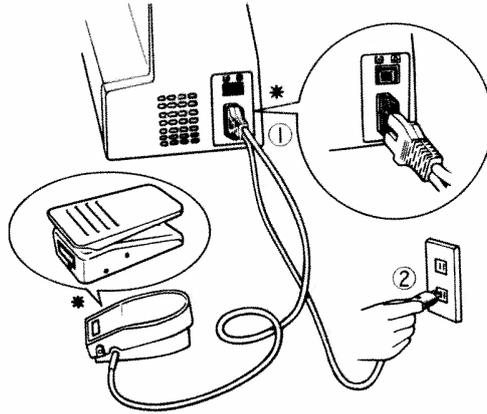
Switch on power to put on machine and turn on sewing light.
