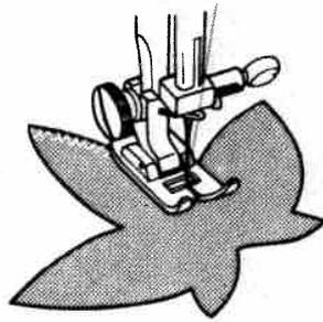
To change direction at corners, or to sew very small circles, stop machine, positioning needle just away from edge of cut-out, lift presser foot and turn material. Lower presser foot and continue sewing.
