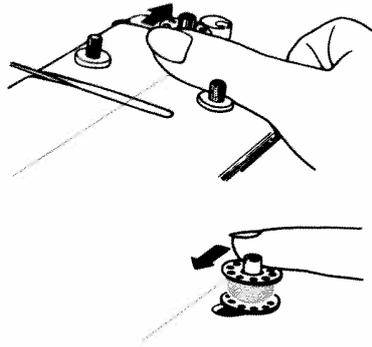
Take off bobbin from spindle and cut thread.
