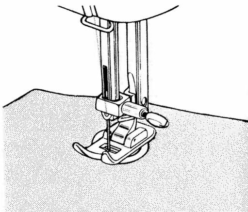
Stop machine when needle is in upper position.
