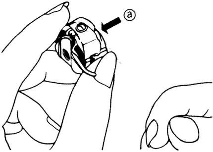
Pulling thread to left, bring it under tension spring then to delivery eye (b).
